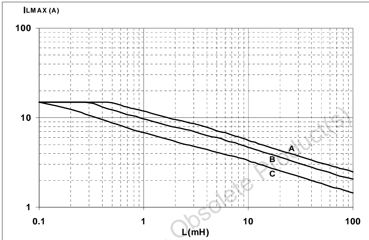
Figure 27. Maximum turn off current versus load inductance
