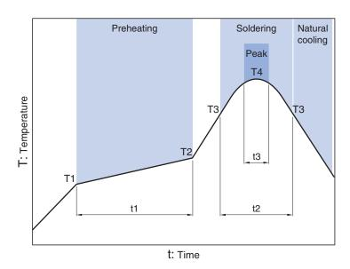
Preheating Soldering Peak Temp. Temp. Time Temp. Time Time T2 T3 T4 t3 150°C 180°C 60 to 120s 230°C 30s 260°C 10s
