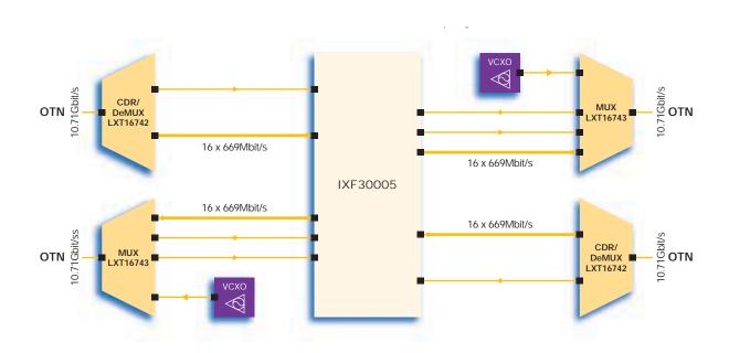
The IXF30005 Wrapper/FEC may be operated as Intra Domain Interface (IaDI) and Inter Domain Interface (IrDI) within an OTN according to G.709, acting as a gateway between two OTNs or as a network node within an OTN. Because of the various types of framing it supports, the IXF30005 may also act as a gateway between existing IXF30001-based network and an G.709 compliant OTN.
