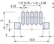
Note) The zero point is the center of mounting.
