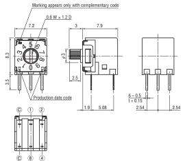
Unless otherwise specified, tolerance:  $\pm 0.3$  (Unit: mm)
