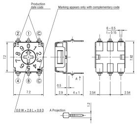
Unless otherwise specified, tolerance:  $\pm 0.3$  (Unit: mm)
