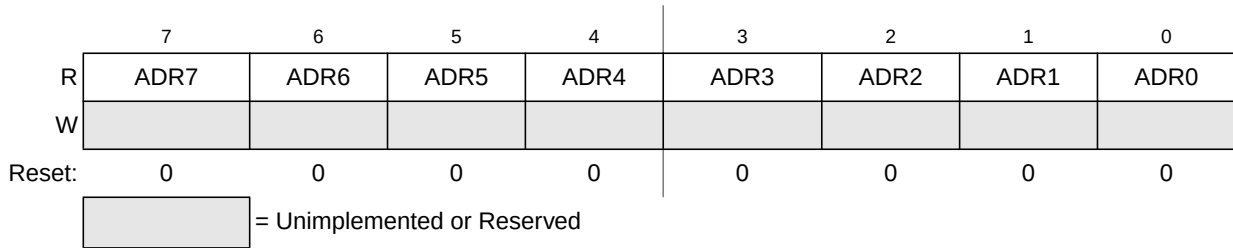
Figure 9-6. Data Result Low Register (ADCRL)
