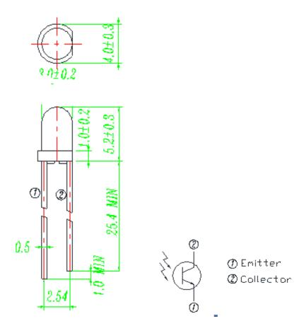
Note: Tolerances unless dimensions ±0.25mm
