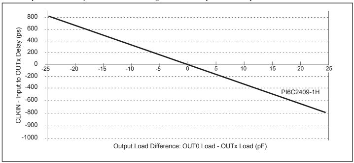
The relationship between loading of the OUT0 signal and other outputs determines the input-output delay. Zero delay is achieved when all outputs, including feedback, are loaded equally.
