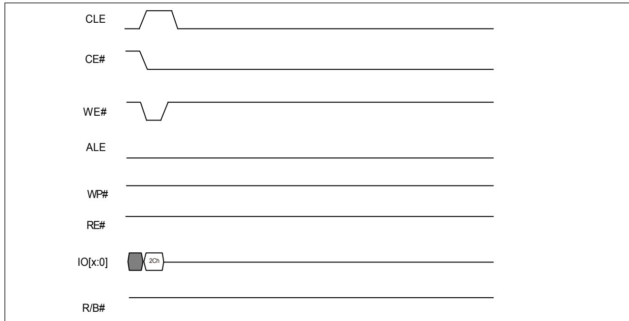
Figure 40. AC Waveforms for Block Solid-Protect
