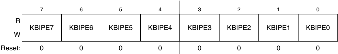
Figure 12-4. KBI Pin Enable Register
