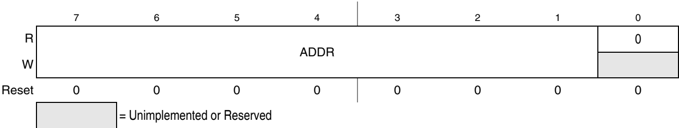
Figure 11-3. IIC Address Register (IICA)
