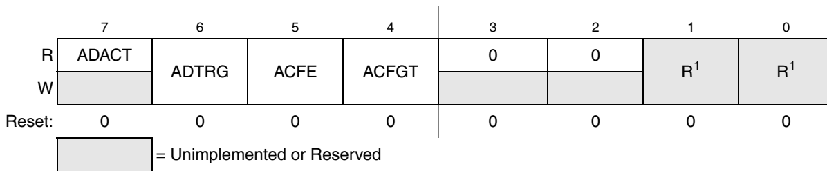
Figure 9-5. Status and Control Register 2 (ADCSC2)
