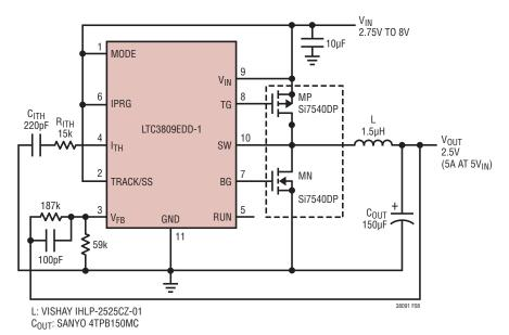
Figure 8. 550kHz, Synchronous DC/DC Converter with Internal Soft-Start
