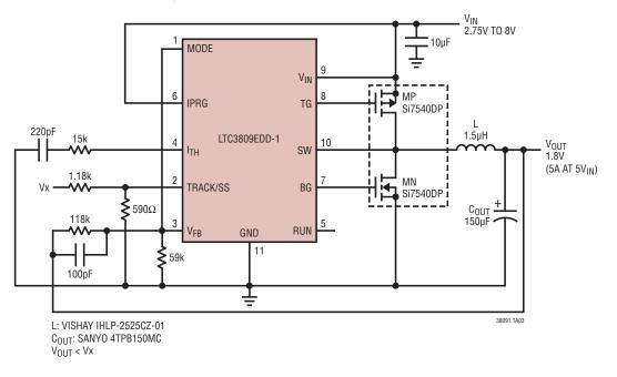
Synchronous DC/DC Converter with Output Tracking
