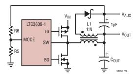
Figure 6. Auxiliary Output Loop Connection
