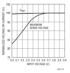
Figure 7. Line Regulation of  $V_{\text{REF}}$  and Maximum Sense Voltage
