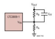
Figure 3. Setting Output Voltage
