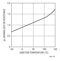
Figure 2. R<sub>DS(ON)</sub> vs Temperature
