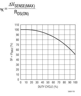
Figure 1. Maximum Peak Current vs Duty Cycle
