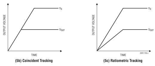
Figure 5b and 5c. Two Different Modes of Output Voltage Tracking
