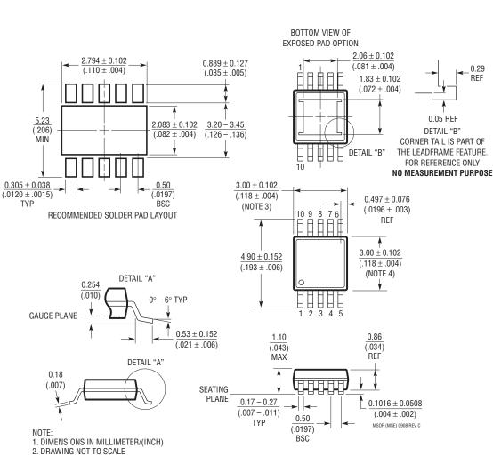
**MSE Package** 10-Lead Plastic MSOP, Exposed Die Pad (Reference LTC DWG # 05-08-1664 Rev C)
