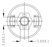
Notes: (1) All dimensions are in mm. (2) Drawing not to scale. (3) Collimator material is PC.
