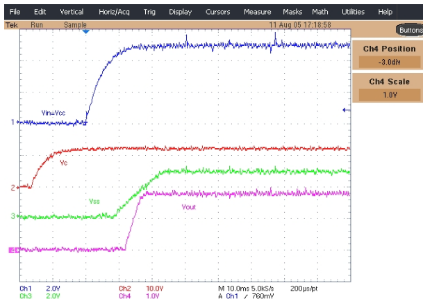
Figure 14 - Start up waveforms Ch1: Vin=Vcc, Ch2:Vc, Ch3:Vss, Ch4: Vout
