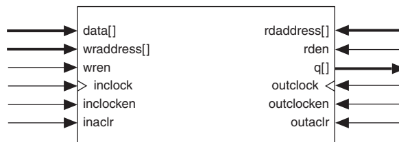
Figure 2-13. Simple Dual-Port and Single-Port Memory Configurations
