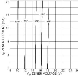
Fig. 4 Typical Zener Breakdown Characteristics
