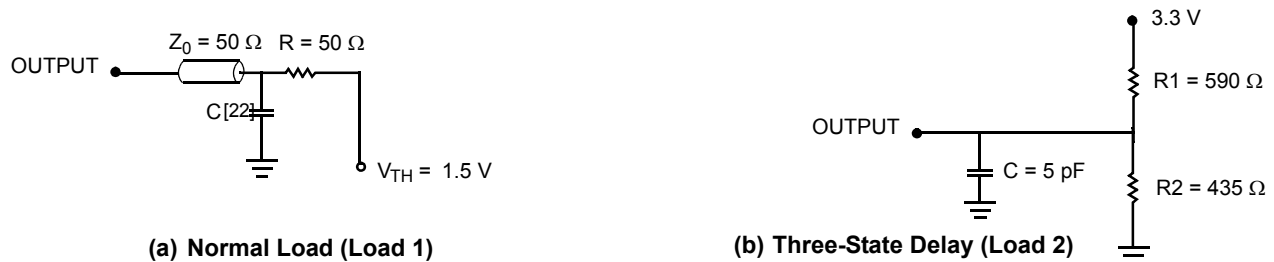
Figure 3. AC Test Loads and Waveforms
