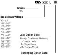
(Blank) = Bulk (Applies to Core Devices Only) TR = Tape & Reel
