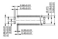
Recommended metal mask pattern Metal mask thickness: When 120µm (Terminal opening ratio: 60%) (Metal-part opening ratio: 100%)
