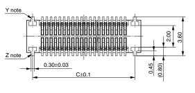
Note: Since the soldering terminals\* has a single-piece construction, sections Y and Z are electrically connected.
