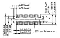
Recommended metal mask pattern Metal mask thickness: When 150μm (Terminal opening ratio: 48%) (Metal-part opening ratio: 100%)
