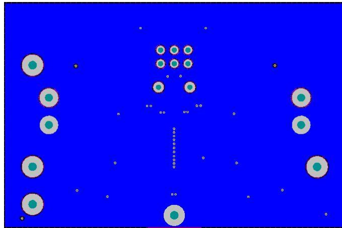
Figure 2. PCB Copper Layout & Silk Screen – Bottom
