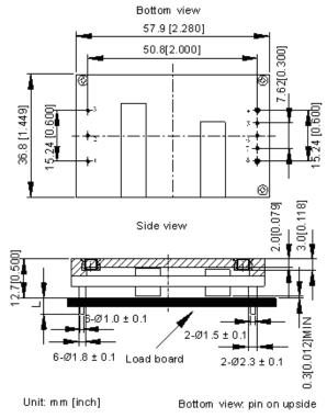
Tolerance: X.Xmm ± 0.5mm [X.X in. ± 0.02in.] X.XXmm ± 0.25mm [X.XX in. ± 0.01in.]
