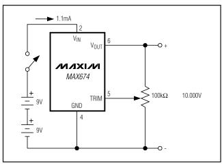
Figure 2. Precision Calibration Standard
