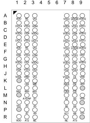
DDR2 SDRAM (128Mx16) LF-BGA Ball-out (Top-View) (10.5mm x 13.5mm Body, 0.8mm pitch)
