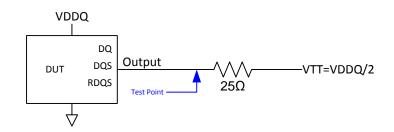
Output slew rate for falling and rising edges is measured between VTT - 250 mV and VTT + 250 mV for single ended signals. For differential signals (e.g. DQS - DQS#) output slew rate is measured between DQS - DQS# = -500 mV and DQS - DQS# = +500 mV. Output slew rate is guaranteed by design, but is not necessarily tested on each device.
