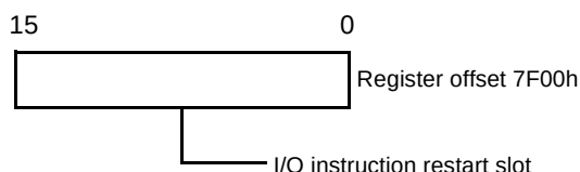
Figure 29. I/O Instruction Restart Register Offset
