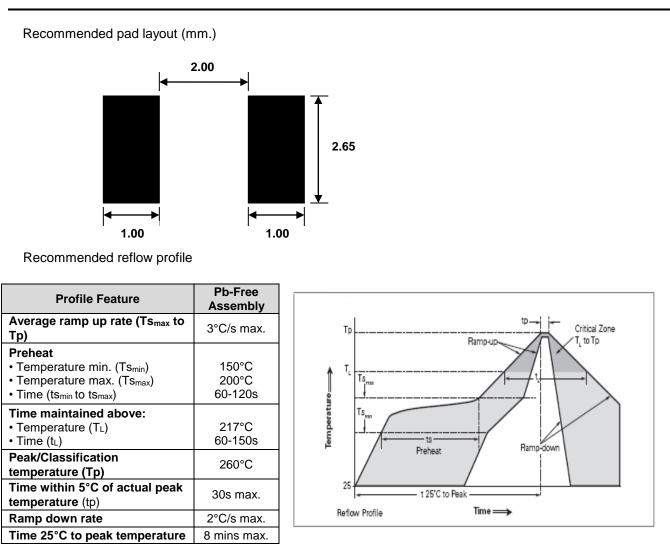
Note: All temperatures refer to top side of the package, measured on the package body surface.
