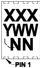
8-Lead DFN (2 x 3 x 0.9 mm)
