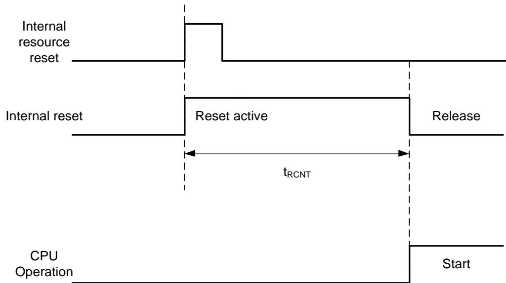
\*: Internal resource reset is not included in return factor by the kind of Low-Power consumption mode.
