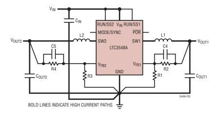
Figure 2. LTC3548A Layout Diagram (See Board Layout Checklist)
