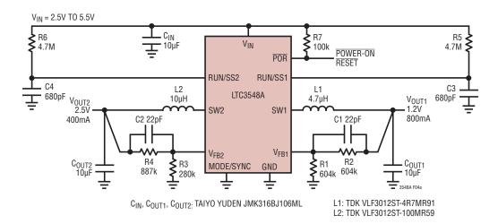
Figure 4. Low Ripple Buck Regulators with Soft-Start
