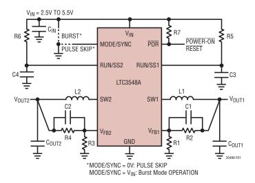
Figure 1. LTC3548A General Schematic
