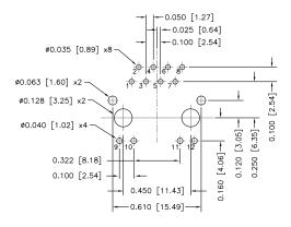
Recommended PCB Layout (Component Side)
