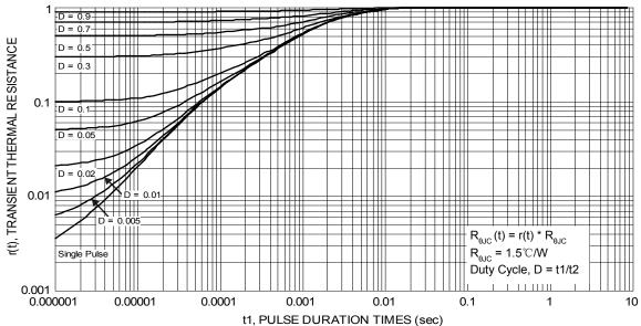
Figure 13 Transient Thermal Resistance
