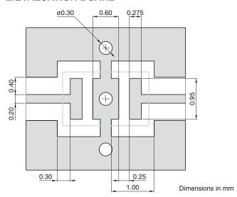
Line width be designed to match  $50\Omega$  characteristic impedance depending on PCB material and thickness.
