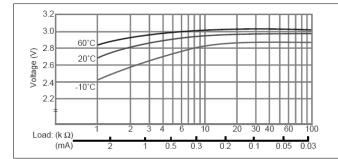
**Operating Voltage vs. load resistance \***
