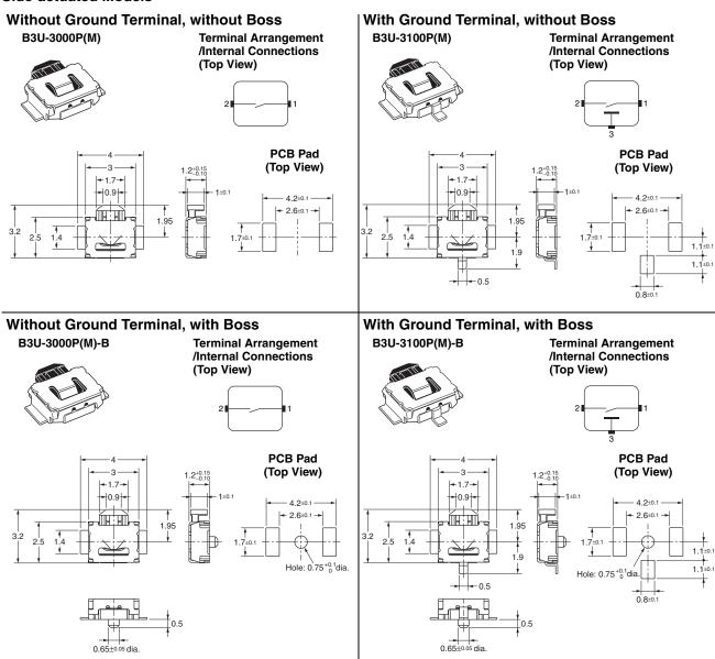
$\textbf{Note:} \quad \text{Unless otherwise specified, a tolerance of $\pm 0.2$ mm applies to all dimensions. No terminal numbers are indicated on the Switches.}$
