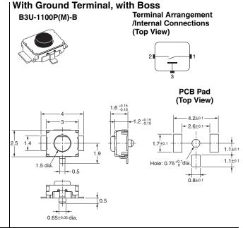
Note: Unless otherwise specified, a tolerance of ±0.2 mm applies to all dimensions. No terminal numbers are indicated on the Switches.
