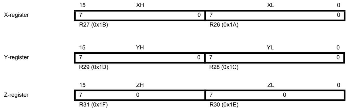
Figure 6-3. The X-, Y-, and Z-registers
