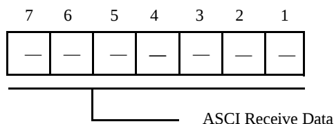
Figure 31. ASCII Receive Register Channel 1R
