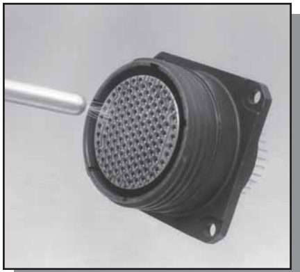
Electrostatic Discharge (ESD) Testing on Tri-Start Filter Connector
