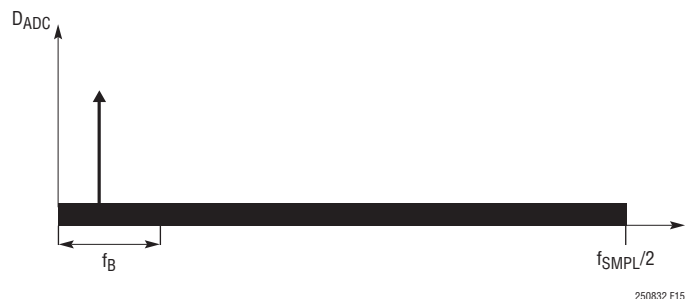
Figure 15. Frequency Spectrum of SAR ADC Core Output
