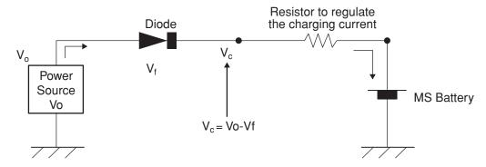
A resistor must be inserted to regulate the charging current, because our rechargeable batteries have a limit for charging current.
