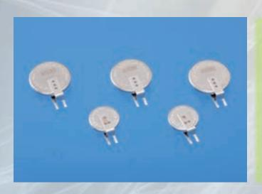
Designed with SII's unique sealing technology, "MS920T" offers a wider operating temperature range than conventional models, while maintaining the features of current MS-series. The conventional MS rechargeable batteries have an operating temperature range up to 60°C. The new MS920T can operate at an even higher temperature of up to 85°C. It is a great fit for devices that operate under high temperature environment, and for apparatuses that have high internal temperature.
