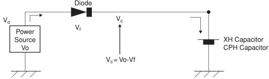
You do not need to insert a resister to regulate charging current.
