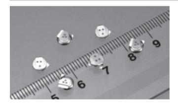
The XH series capacitor has a better discharge characteristic above 3V. It is an environmentally friendly product that is reflow mounted by Pb-free soldering. It features high capacity, and long-term reliability, as well as a wide operating voltage range. It is thus suitable for backup power supply of clock and memory functions on mobile and information devices.
