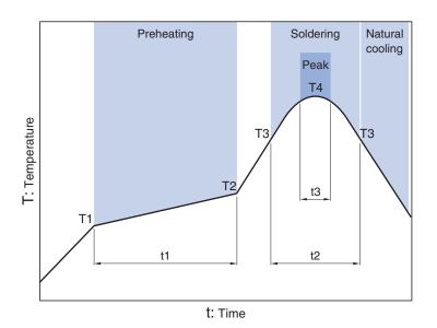
Preheating Soldering Peak Temp. Temp. Time Time Temp. Time T1 T2 **T**4 t1 тз t2 t3 150°C 180°C 60 to 120s 230°C 260°C 10s 30s
