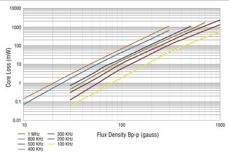
Core Loss vs. Flux Density
