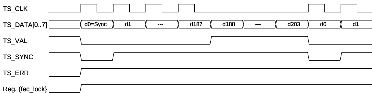
Figure 13. Gapped TS Parallel Mode with Rising Active Clock Edge, Enabled Parity Bytes, and Active Low Polarities
