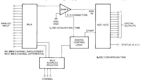
A high speed data acquisition system employing the SHM-6. This system is capable of a 110 kHz throughput rate with 12 bit resolution. In this system the SHM-6 is used with DATEL's ADC-HZ12, a high-speed hybrid 12 bit A/D converter, and DATEL's MV-808, a low cost monolithic analog multiplexer. Use of a low on-resistance MUX is recommended, so that the time constant formed by MUX on-resistance and bus capacitance does not limit the acquisition performance of the SHM-6.
