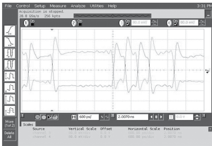
Data Waveforms, 2.5Gbps (left) & 5.0Gbps (right)
