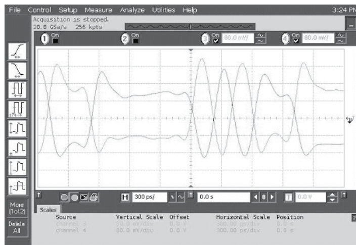
Data Waveforms, 2.5Gbps (left) & 5.0Gbps (right)
