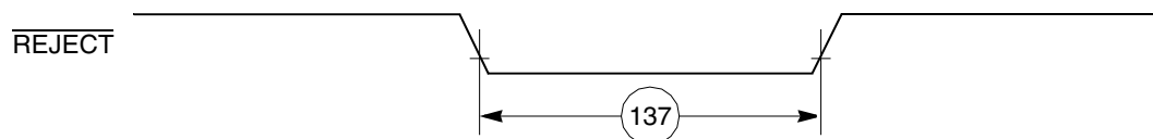
Figure 63. CAM Interface \overline{\text{REJECT}} Timing Diagram
