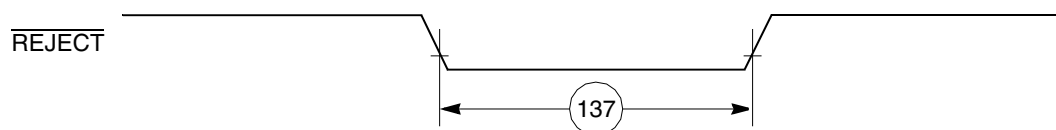
Figure 63. CAM Interface \overline{\text{REJECT}} Timing Diagram
